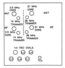
Reference: Layout of ANT. and RF Coil trimmers in RF Unit UC-1117J.
